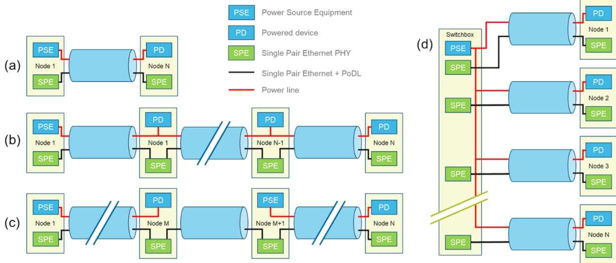
Figure 3: Network topologies hybrid connector: (a) Point to point, (b) Bus powered, (c) Bus powered with additional resupply points, (d) Switch with hybrid power source
