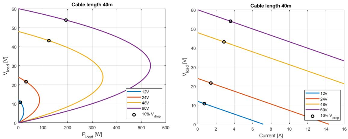
Figure 2: Voltage drop over the AWG 18 copper wire as function of transmitted power and current.
