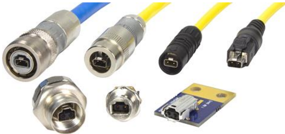
Picture 4: SPE connector versions according to IEC 63171-6 as IP65/67 as well as IP20 versions (top row from left to right: M12 PushPull Stvb., M8 PushPull Stvb., M8 SnapIn Stvb. and IP20 Stvb. / bottom row from left to right: M12 socket with screw and PushPull locking, M8 socket with SnapIn and PushPull locking, angled IP20 PCB socket) (Source: HARTING)
